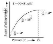
The plot between the extent of adsorption (m) against the pressure of gas (*P*) at constant temperature (T) is called the adsorption isotherm.
